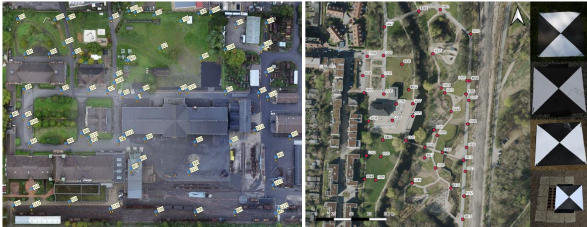
Fig. 3: GCP overview for UAV test field Zollern colliery (left, Source: Bäumker 2020) - and UAV test field Inseipark Hamburg-Wilhelmsburg (centre), and GCP targets on different surfaces (right) - grass, asphalt, sand and stone (Kersten et al. 2022)
