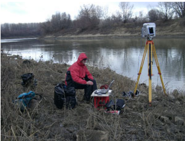
Fig. 14: Scanner and equipment in use at the river Tisza
