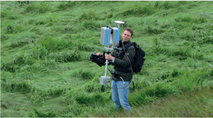
▲ Figure 2, Scanning while walking using the kinematic laser scanning system from the company p3d systems.
