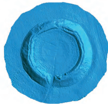
▲ Figure 4, The mesh from the UAS data, filtered to a 20cm grid cell using the lowest point.
