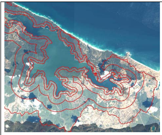
Figure 2. Drinking water basin with different protection zones
