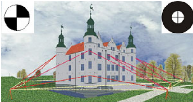
Fig. 3: Geodetic control point determination and signalisation of control points (upper left and right corner)
